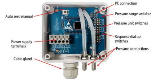
Figure 4 LFM11X-XE(F)X Internal Circuit
